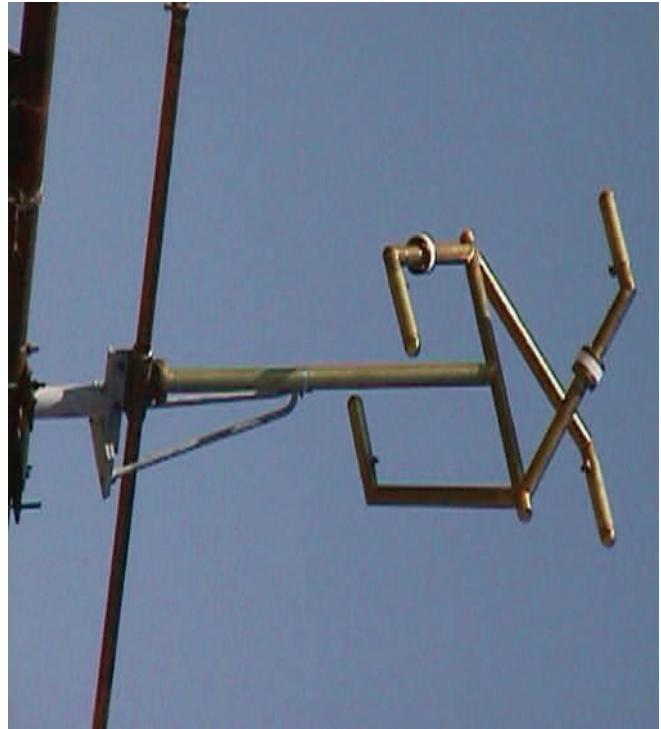
This antenna is designed with the same principles as JAMPRO's patented PENETRATOR series of FM antennas, which set the industry standard for FM side mount antennas. The shunt fed design eliminates the need to "slug tune" the antenna in the field for optimum performance. Unlike similar, older designs, the Optimizer uses low impedance bays for un-excelled stability and band pass.
