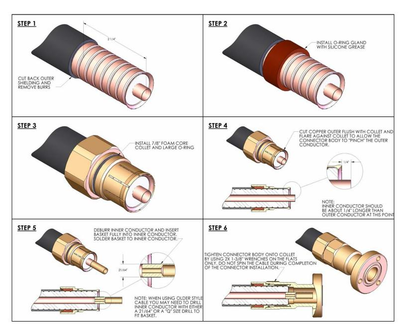
Pressure test cable and connectors to ensure proper installation of connections. Congratulations, you have completed installation of the 7/8" EIA foam cable connector.
