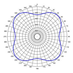
Standard Omni Azimuth Pattern
